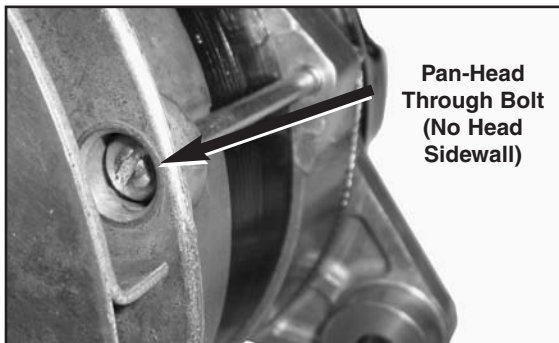
Figure 4 - Through Bolt Head Inspection Example Shown.
