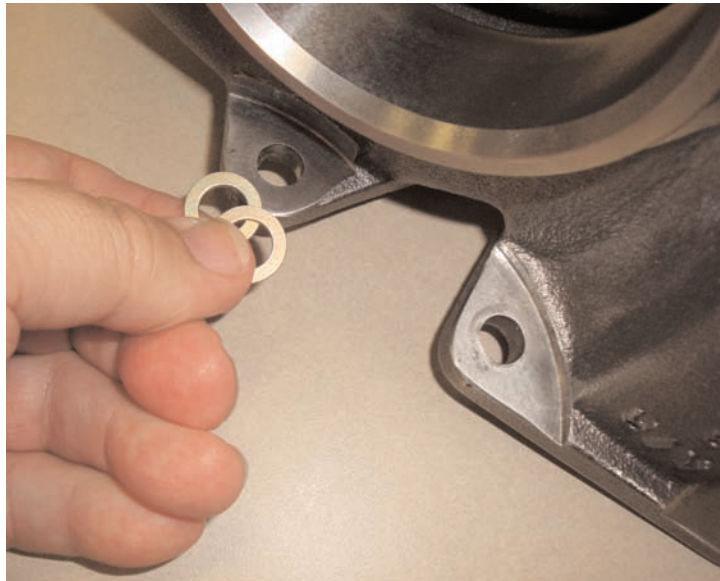
Figure 4 - Shimming at Turbine Housing Mounting Tab
