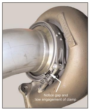
Figure 2 - "V" band Clamp Showing Gap
