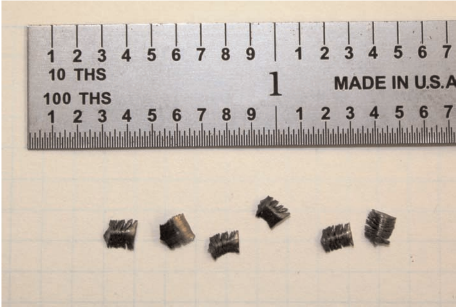
Fig. 2 - Typical Burrs as Removed from Hex Key Socket
